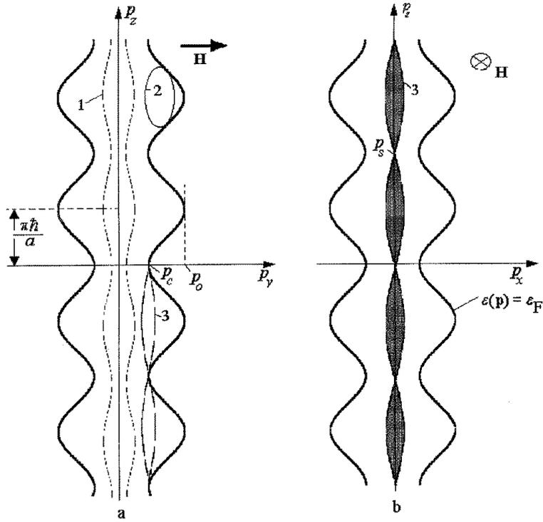
Figure 1: Different types of electron trajectories in the momentum space in a magnetic field applied parallel to the layers: 1, an open trajectory; 2, a closed orbit; 3, the self-intersecting orbit containing the saddle points  $\mathbf{p}_s$ . The cross-section  $p_y = p_c$  separates the region of open cross-sections from the closed ones.
