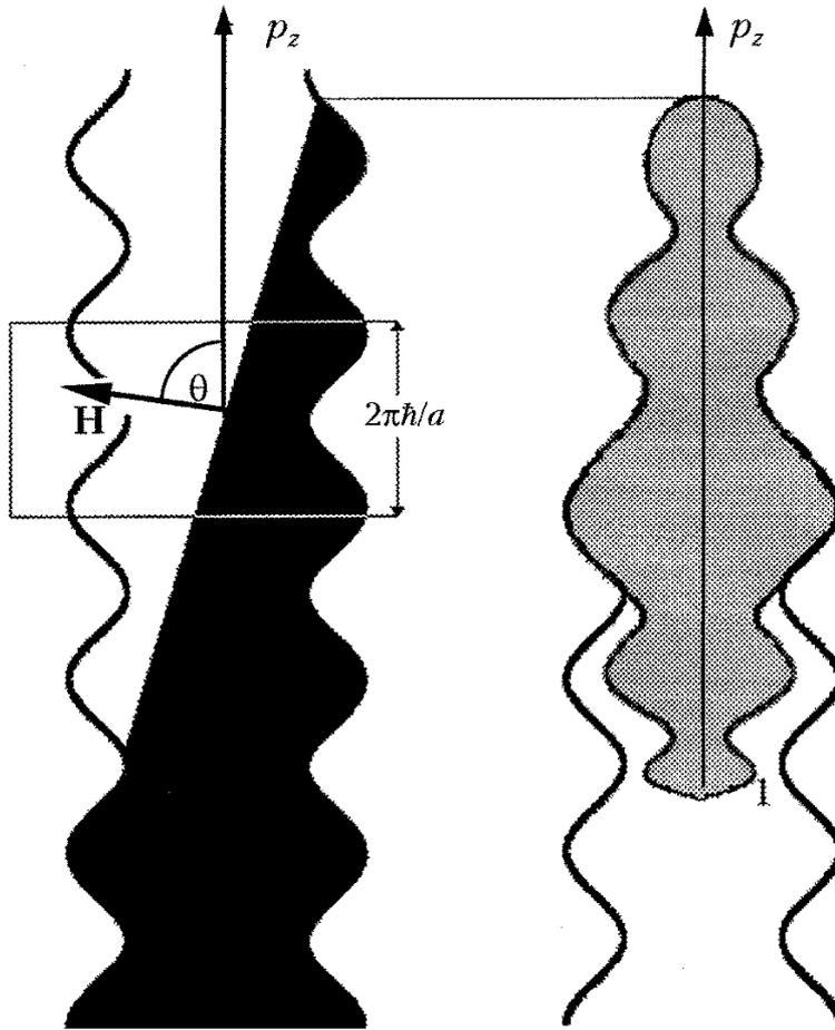
Figure 2: Electron trajectories on the Fermi surface in an oblique magnetic field ( $\theta$  is the angle of deviation of the vector  $\mathbf{H}$  from the layers-plane). An electron orbit (1) passes through a few number of cells in the momentum space.
