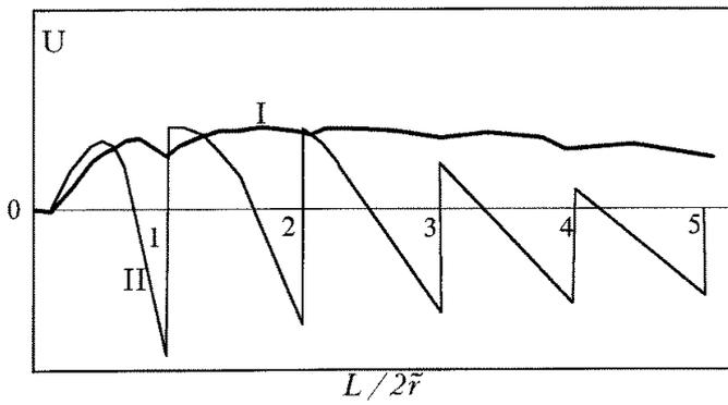
Figure 11: Experimental geometry (a) and the shape of the transverse ( $L \perp H$ ) electron focusing signal (curve I) and its derivative with respect to  $H$  (curve II) in the case when the line  $L$  connecting the contacts on the same face of the sample and the magnetic field vector  $H$  lies in the plane of the layers.
