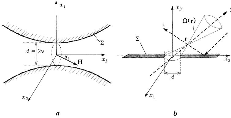
Figure 13: A model of the point-contact in the form of a single-sheet hyperboloid of revolution (a); its limiting case ( $\beta = 0$ ) is a circular orifice (b);  $\Omega(\mathbf{r})$  is the solid angle within which velocities of the electrons passing the contact along the ballistic trajectories fit.
