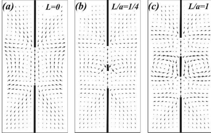
Fig. 3. Current distribution pattern in the vicinity of a double point contact between two  $d$ -wave superconductors in the absence of a transport supercurrent ( $v_s = 0$ ) and at the phase difference  $\phi = \pi/2$ .
