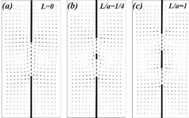
Fig. 2. Current distribution pattern in the vicinity of a double point contact between two conventional superconductors in the presence of a transport supercurrent ( $v_s \neq 0$ ) and at the phase difference  $\phi = \pi$ .
