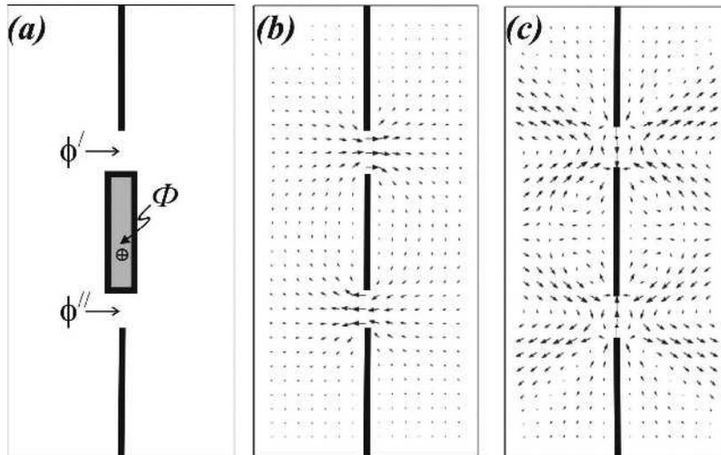
Fig. 5. Double point contact with the phase difference at one orifice  $\phi'$  being not equal to the phase difference at the other orifice  $\phi''$ : (a) scheme, (b) and (c) current distribution pattern for the contact of conventional and  $d$ -wave superconductors respectively, at  $\phi' = -\phi'' = \pi/2$ .
