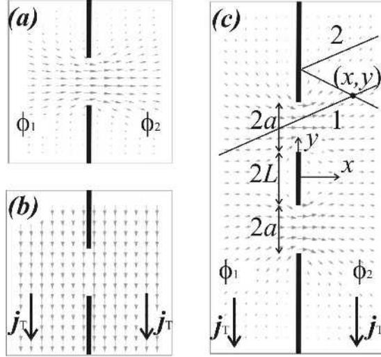
Fig. 1. Models of a single point contact (a,b) and double point contact (c) between two superconductors with different phases of the order parameter,  $\phi_1$  and  $\phi_2$  (a) and with homogeneous transport supercurrent  $j_T(v_s)$  in the banks. The current distributions are shown when either the phase difference is present (in the absence of a transport supercurrent) (a,c) or when the transport supercurrent is present (b).
