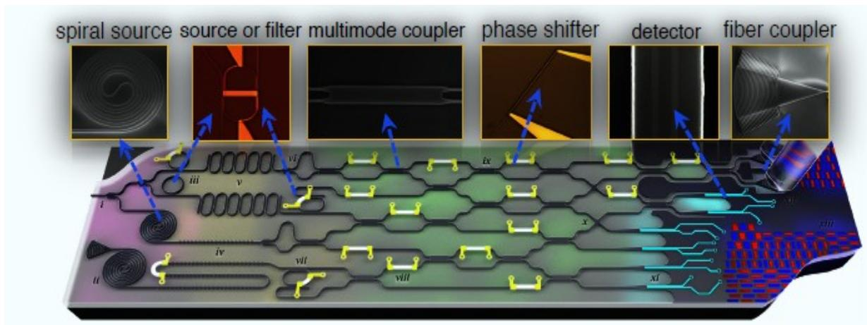
Fig.1. How a complete integrated quantum photonic circuit will probably look like in the next few years (from [2]). From left to right: photon pairs produced by spiral waveguides will be filtered from the intense pump which generates them and subsequently coherently manipulated by a complex network of reconfigurable splitters and phase shifters. These optical qubits will be detected at the output of the circuit to form the result of the computation.
