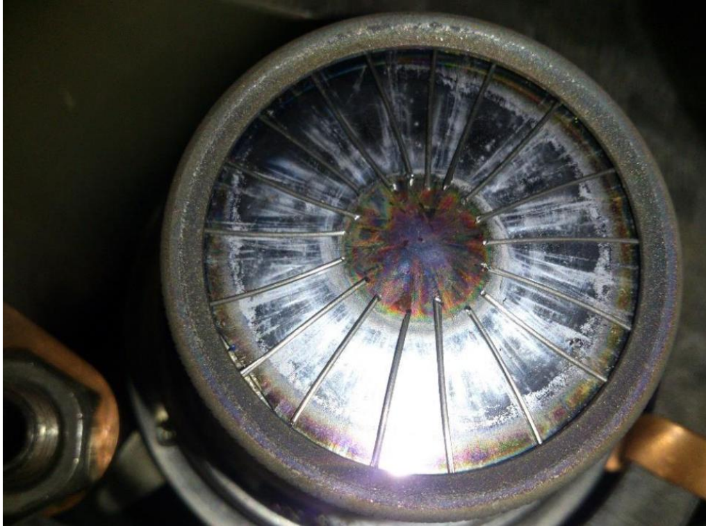
Fig.2 . Magnetron for sputtering Si(W), complex target consists of a silicon plate with tungsten wires located on it.
