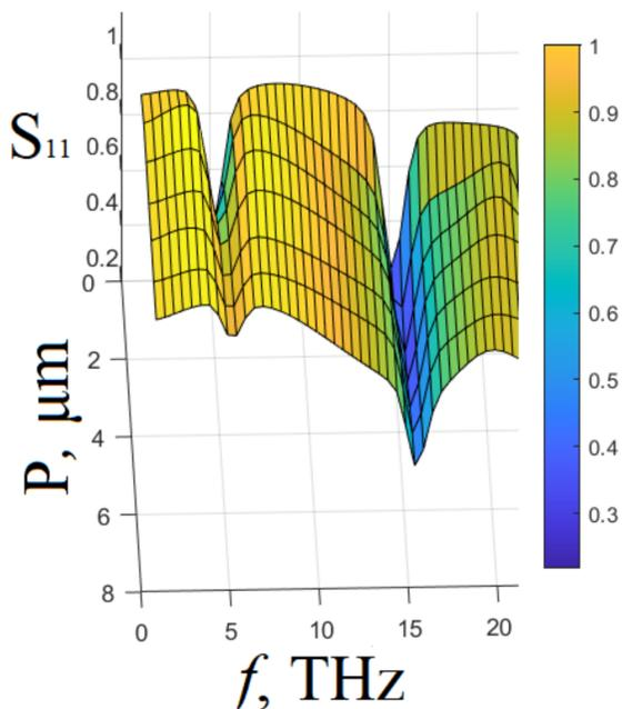
**Fig. 2.** The reflection coefficient  $S_{11}$  as a function of frequency  $f$  and distance between neighboring graphene strips  $P$ .
