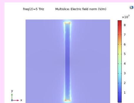
**Fig. 3.** Electric field distribution in metasurface unit cell at 5 THz.
