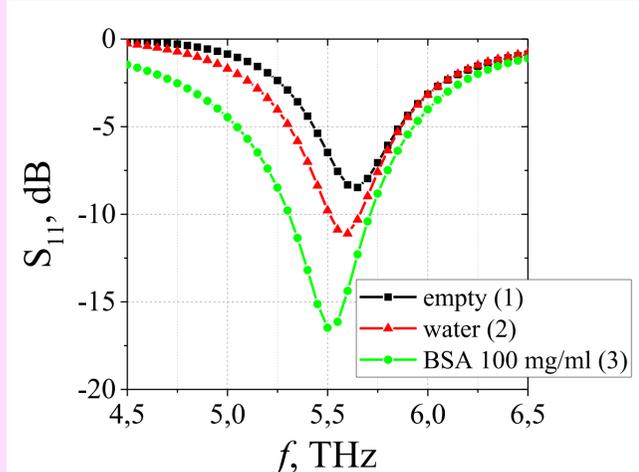
**Fig. 4.** The behaviour of reflection coefficient  $S_{11}$  of the graphene-based metasurfaces with different analyte layers: (1) no analyte, (2) water layer, (3) 100 mg/mL BSA aqueous solution.
