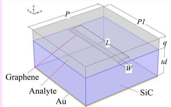
**Fig. 1.** The unit cell of the graphene-based metasurface, consisting of SiC layer ( $td = 2.5 \mu\text{m}$ ) with a centrally positioned graphene strip,  $W = 0.4 \mu\text{m}$ ,  $L = 6.36 \mu\text{m}$ .
