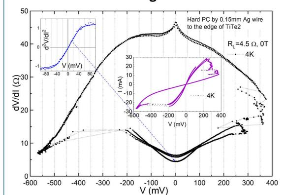
Fig.3. Resistive switching in  $dV/dI(V)$  for  $\text{TiTe}_2$  PC by „clock wise“ V-sweeping. Central inset:  $I-V-C$  of the same PC. Left inset: calculated  $d^2V/dI^2$  of low-resistance state for the same PC.
