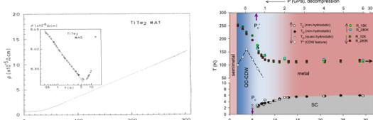
Electrical resistivity of  $\text{TiTe}_2$  single crystals. Y. Koike *et al.*, *JPSJ* 52, 597 (1983)
