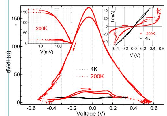
Fig.4. Resistive switching in  $dV/dI(V)$  for  $\text{TiTe}_2$ -Ag “hard” PC at two temperatures. Inset (right):  $I(V)$  curves for this PC. Inset (left):  $dV/dI(V)$  in log-scale
