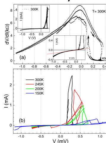
Fig.2. a)  $dV/dI(V)$  and  $I(V)$  curves (insets) at 300K with “diode”-like effect for  $\text{TiTe}_2$  “soft” PC. (b)  $I(V)$  curves for another soft PC at  $T=300 \rightarrow 150$ K.
