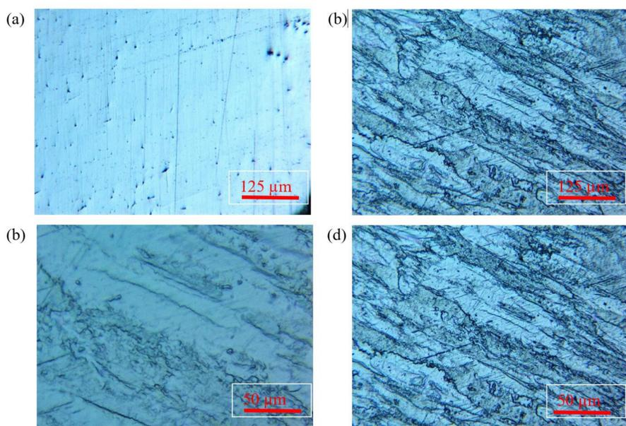
Fig. 1. Metallographic images of  $\text{Mo}_{48}\text{Re}_{52}$  foil before (a)–(c) and after the HPT treatment (a) and (d). The polished surface is the same for both cases (a). The surfaces after etching with 35% nitric acid for the original sample at two scales (b) and (c), and for the HPT treatment sample (d).
