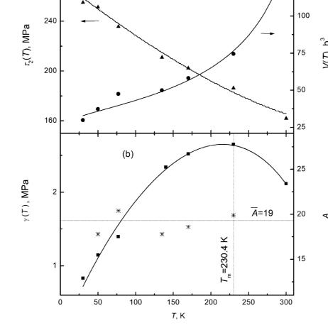
Temperature dependences of plasticity characteristics in state (I) at  $\epsilon$ =0.02: (a)  $\blacktriangle$  – yield stress  $\tau_2(T)$  and  $\bullet$  - activation volume of the plastic deformation process V(T); (b)  $\blacksquare$  - speed sensitivity of deformation stress  $\gamma(T)$  and  $^*$  - empirical values of parameter A. In both figures, solid lines show analytical approximations of experimental points by theoretical formulas.
