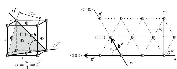
$\{111\}$ <110> slip system and straight dislocations in an fcc crystal: (a) – unit cell; (b) – one of the sliding planes  $\{111\}$ .
