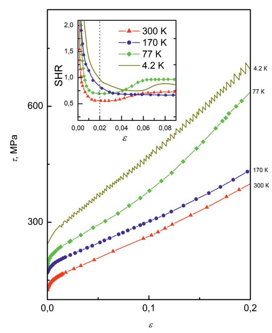
Diagrams of compression deformation of the alloy  $AI_{0.5}CoCrCuFeNi$  in " $\tau-\epsilon$ " coordinates at different deformation temperatures in structural state (I) [3].
