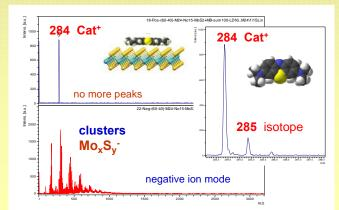
In the LDI mass spectra of the (MB-MoS<sub>2</sub>) dry sample, recorded in positive ion mode, a single abundant peaks envelope with isotopic distribution characteristic of intact cation of MB+ was present. This feature correlates with the monomeric adsorption of MB<sup>+</sup> cations on the nanostructured surfaces.
