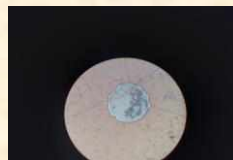
Fig. 4. Appearance of a non-uniform cathode film (a bright spot with a diameter of about 0.5 mm) on niobium oxide after its combined breakdown in a circuit with a 180 \mu F capacitor and a limiting resistance of 1 kOhm with a discharge resistance of 10 Ohms.
