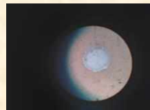
Fig. 5. Appearance of a homogeneous cathode film (a bright spot with a diameter of about 0.5 mm) on niobium oxide after its combined breakdown in a circuit with a 180 \mu F capacitor with a discharge resistance of 20 Ohms and a limiting resistance of 1 kOhm.
