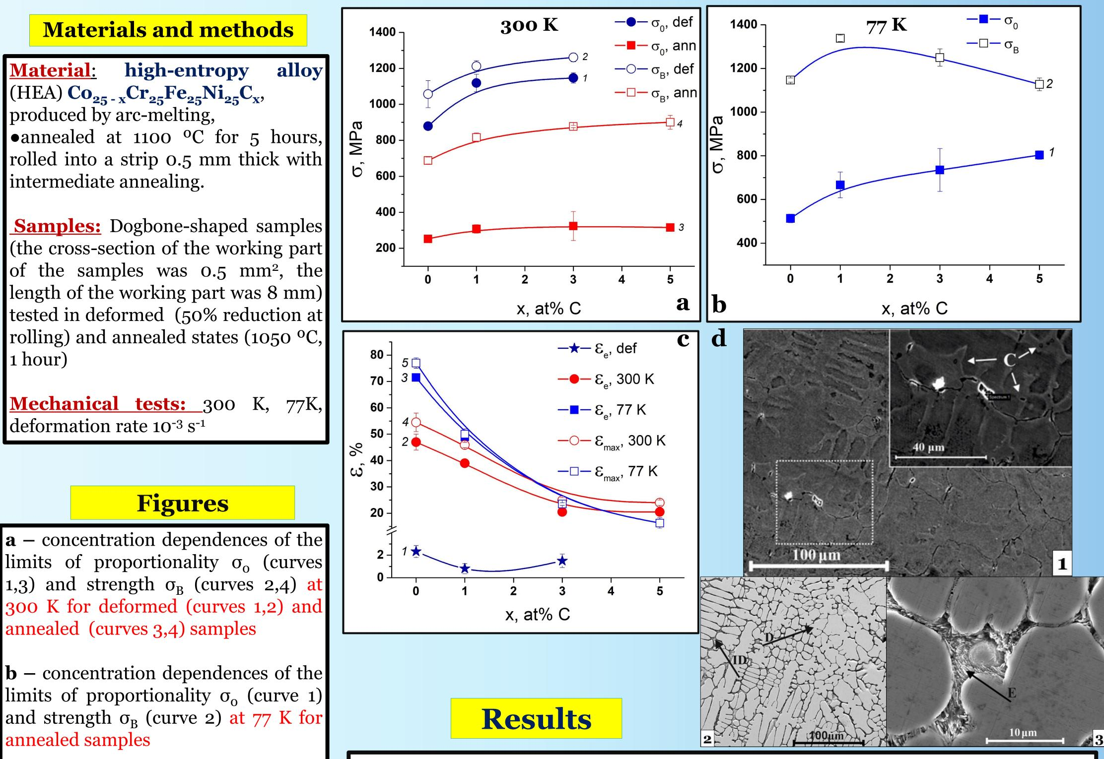
of the samples was 0.5 mm<sup>2</sup>, the length of the working part was 8 mm) tested in deformed (50% reduction at rolling) and annealed states (1050 °C, 1 hour)
