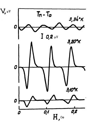
Voltage oscillations in a superconducting interferometer in the resistive state with variation of the external magnetic field in the absence of transport current through the interferometer.
