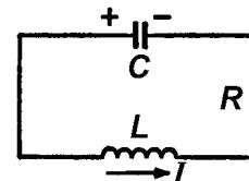
$$IR = \varphi_1 - \varphi_2 + \Theta_c \quad \text{или} \quad IR = -\frac{q}{C} - L \frac{dq}{dt},$$
